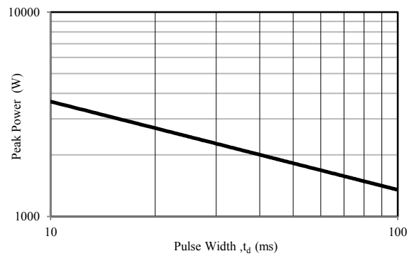
Fig. 4 - Peak Pulse Power Rating Curve
